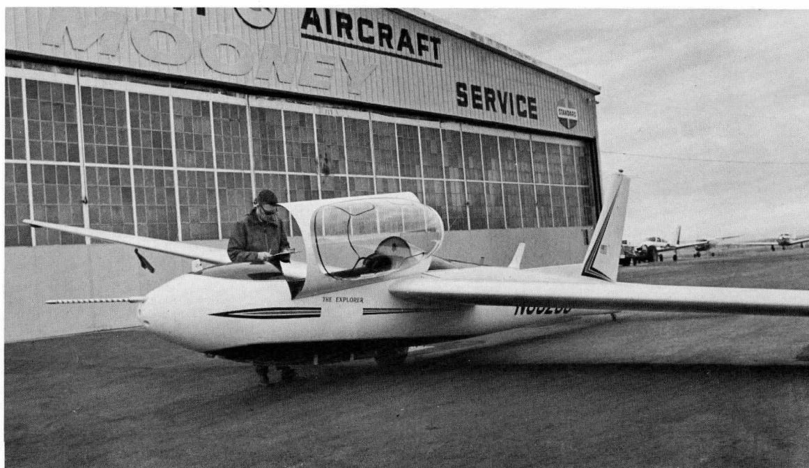
The Schweizer 2-32 is a high-performance, all-metal sailplane with a soaring altitude capability of 15 km. Empty weight is 377 kg, and maximum certified gross weight is 649.2 kg. Length is 8.16 m, and wing span is 17.4 m. Minimum sink (the rate of descent in level flight through still air) is about 1 m/sec and the maximum glide ratio is 30:1 at about 95 km/hr indicated airspeed (at a height of 1 km in still air, it can glide to a landing 30 km away). A two place carrier, it can accommodate an observer, elaborate navigation equipment, and scientific instrumentation.
